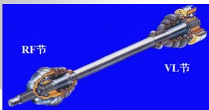
The image shows two types of ball cage joints: RF (Fixed) and VL (Telescopic). The RF joint has a fixed housing, while the VL joint has a telescopic housing that allows for axial movement.
