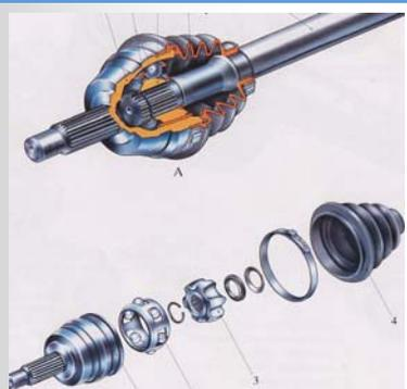
The diagram shows the exploded view of an RF joint with numbered parts: 1. Driving shaft, 2. Steel band, 3. Lock ring, 4. Outer shell.
